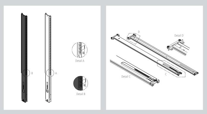
**WIS Item No. 228010002** ADAICO sliding pillar with vertical and internal keyhole recesses, 2,587 to 2,987 mm, cathodic dip-coated, black
