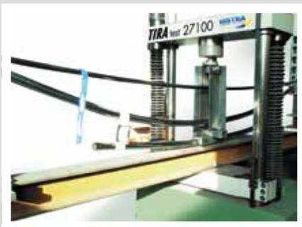
The garment rails are subjected to load carrying tests at regular intervals in the own test facilities.
