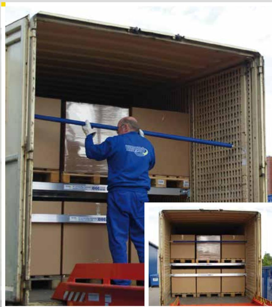
WISTRA double storey systems are manufactured in different versions and can be attached at variable heights.
