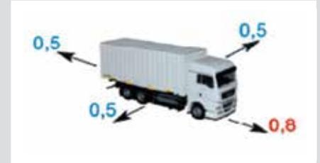
Form-fit (with even loading) according to DIN EN 12195-1:2004/VDI 2700 ff
