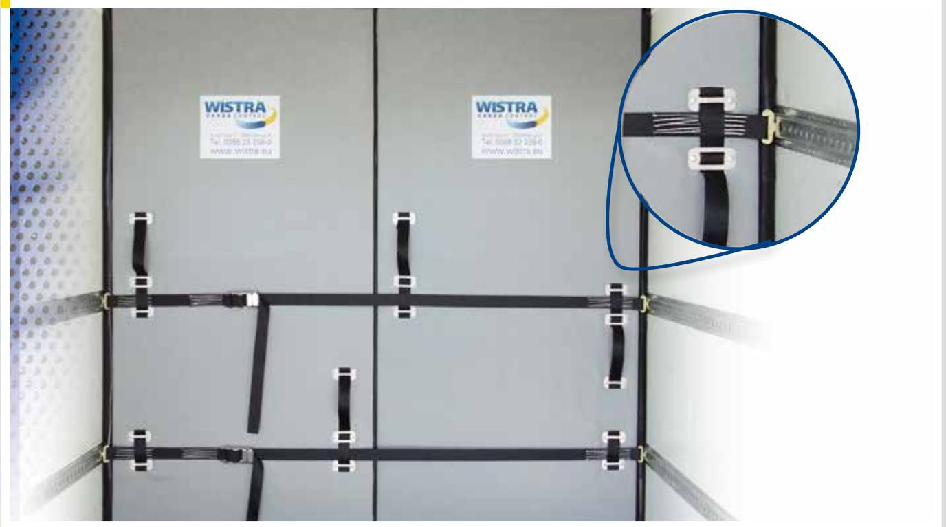
A division is possible for large cold safe walls. The cold safe wall shown here is additionally fixed to the existing lashing tracks.
